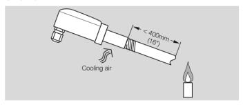
The sensor is mounted to a  $\frac{1}{2}$ " viewing tube using the adapter (supplied) with integrated quartz glass heat guard. The viewing tube should be directed at the first flame third, as this is where the highest UV radiation is generally found. The inside of the steel tube should not be coated
